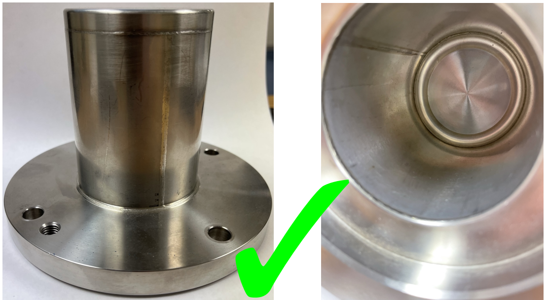
Fig. 13: Containment can Left: Outer surface free from grooves Right: Inside free from grooves
