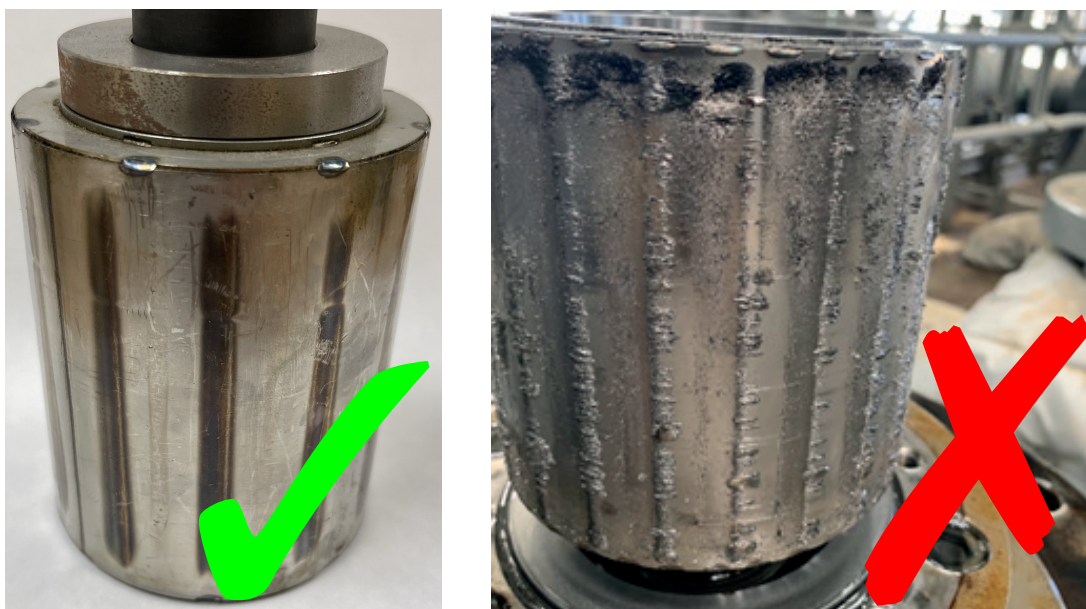
Fig. 15: Inner rotor Left: Inner rotor without adhesions Right: Large amount of iron particles accumulated on the inner rotor
